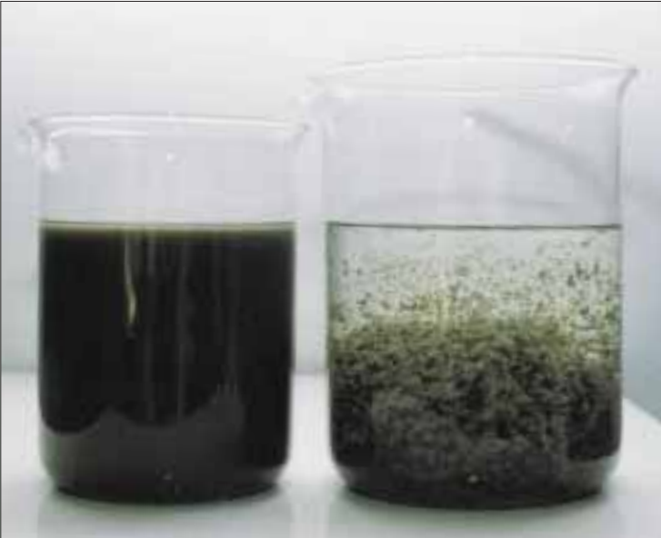
Sludge conditioning with polyelectrolyte
